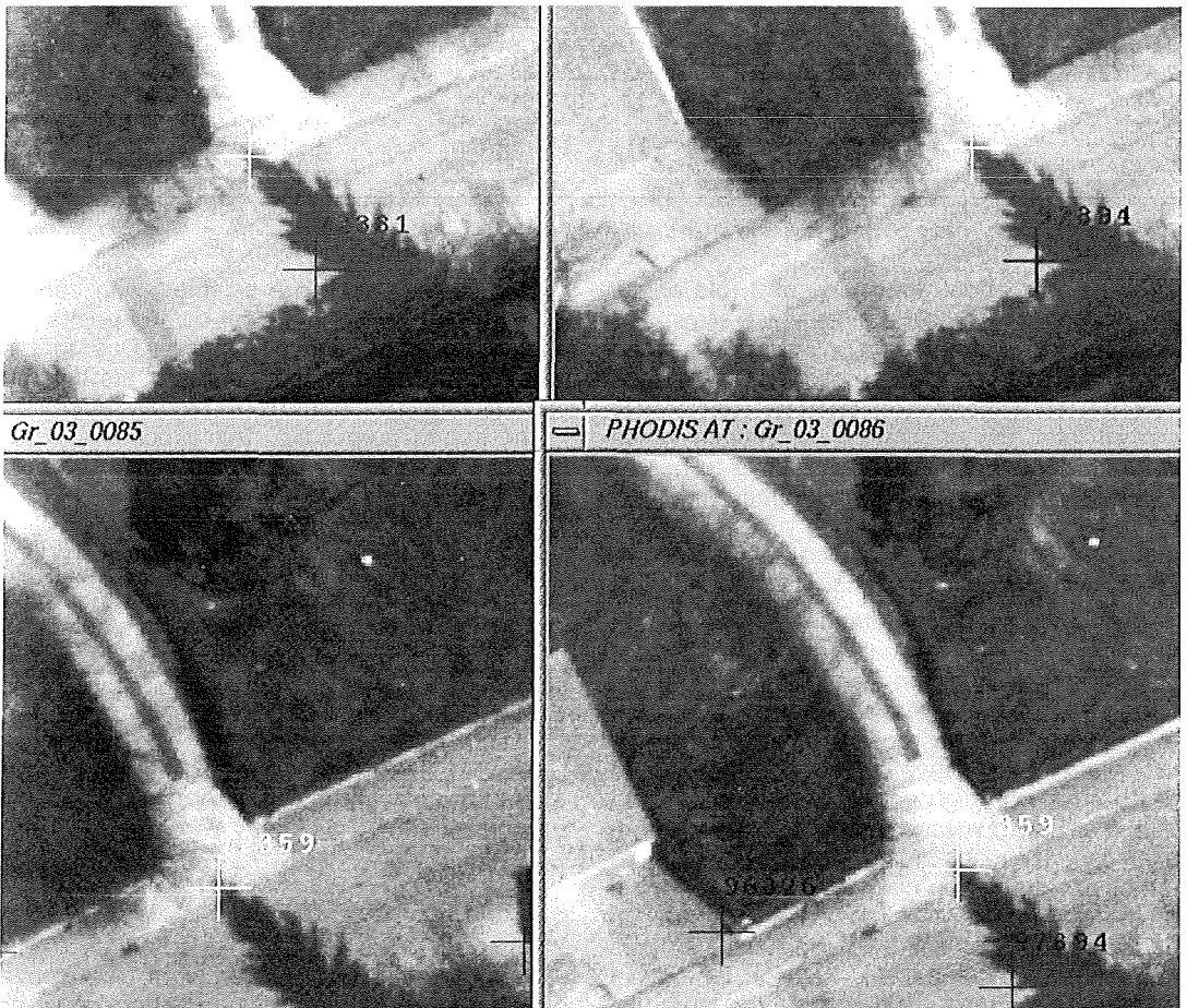
Fig.4: Tie point 72359 is extracted from tree shadows. As we see it was moved in lower strip due to shadow moving, even the feature positions were exact the same location in both strips.
